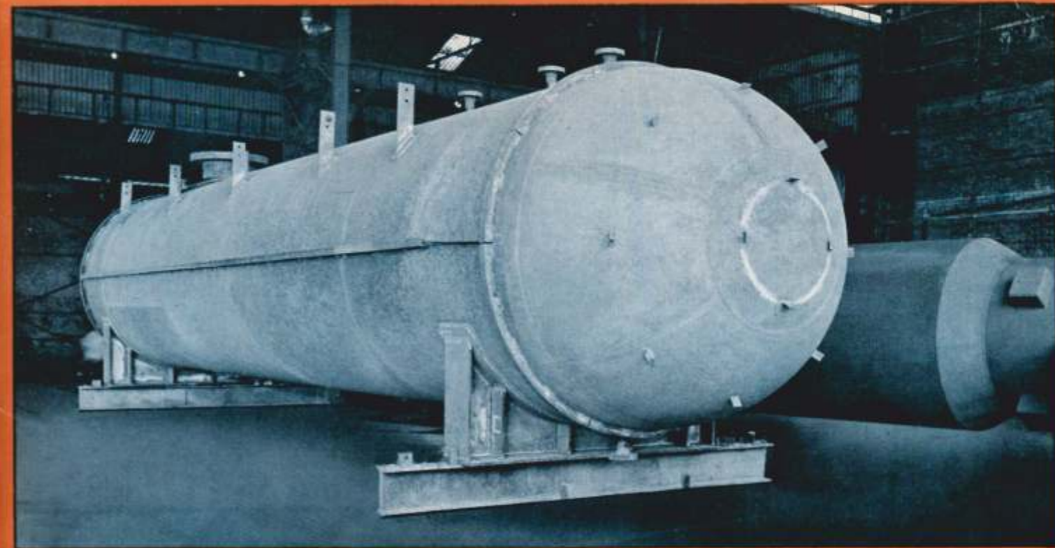
50 M 3 high pressure hydrogen storage vessel for Indian Petrochemicals
